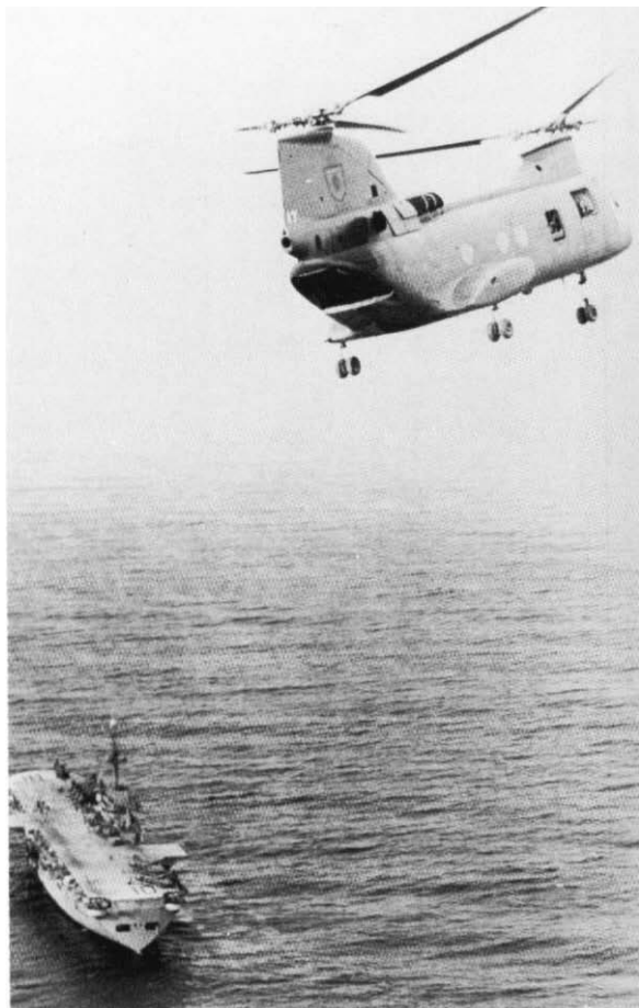
Department of Defense (USMC) Unnumbered Photo A Marine Boeing Vertol CH-46 Sea Knight helicopter from HMM-165 approaches the helicopter carrier USS Tripoli (LPH 10) for a landing. Because of concern for space on board amphibious ships, Marines depended on larger capacity helicopters to carry the assault force so as to require fewer helicopters on board ship.
