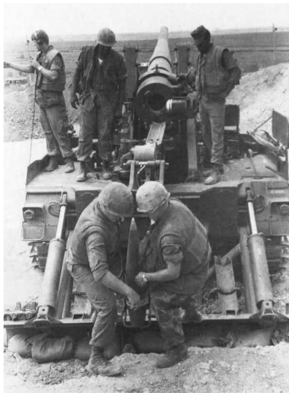
Department of Defense Photo (USMC) A371877 With each round weighing close to 150 pounds, loading a 175mm gun required two Marines. The gun was the largest weapon in the Marine artillery arsenal.
